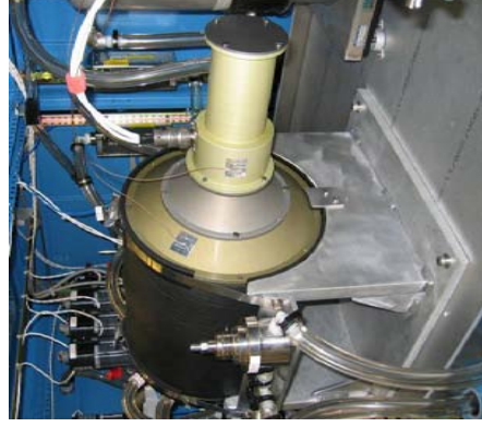
Honeywell's Cascade Distillation Subsystem (CDS) test stand
