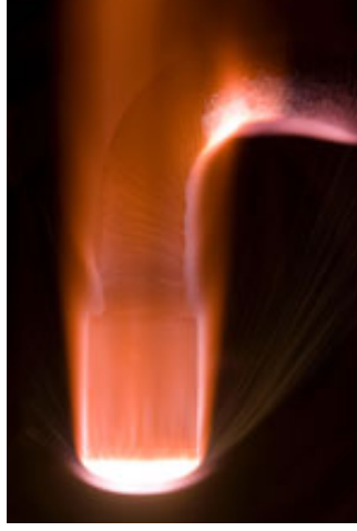
Arcjet testing of TPS material
