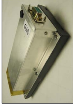
Lithium-ion battery for spacesuit
