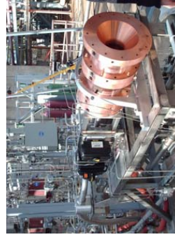
KTE LOX/Methane workhorse main engine installed at MSFC TS500
