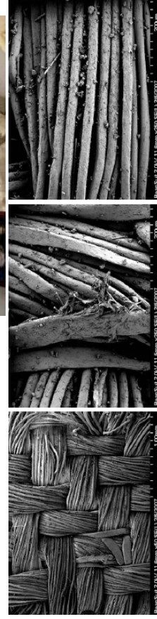
Electron micrographs from GRC showing damage to the outer layer of Alan Bean's Apollo 12 suit
