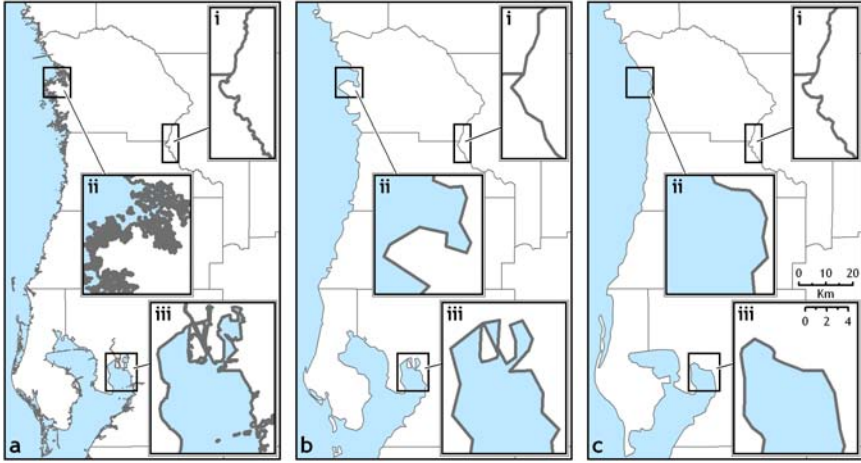
FIGURE 3.8 County boundaries along the Florida Gulf Coast drawn at 1:2,000,000: (a) base data from the Census TIGER files, with inland water extensions clipped, (b) NHGIS generalization for a 1:2,000,000 target scale, and (c) the Census cartographic boundary files. SOURCE: With permission from the NHGIS and Jonathan Schroeder.
