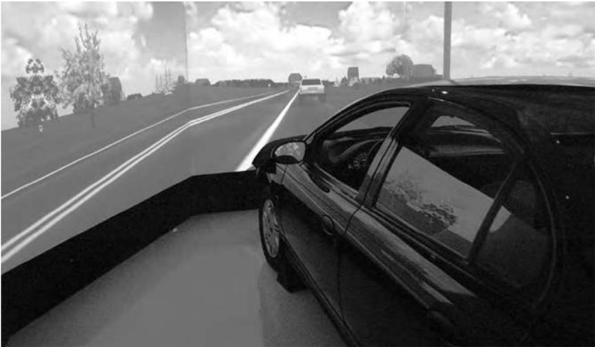
Figure 2.4 A simulated environment photographed from outside the vehicle.
